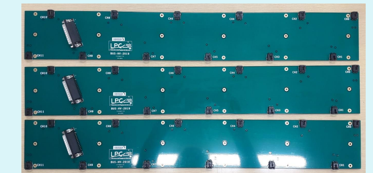
Set of 3 HV Bus prototypes produced this year following the design from LPC Clermont Ferrand
