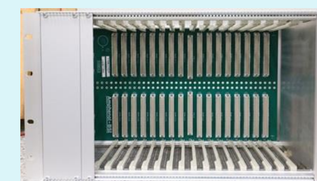
Prototype of the crate for the boards. It has a midplane and the HVremote boards go in the back.
