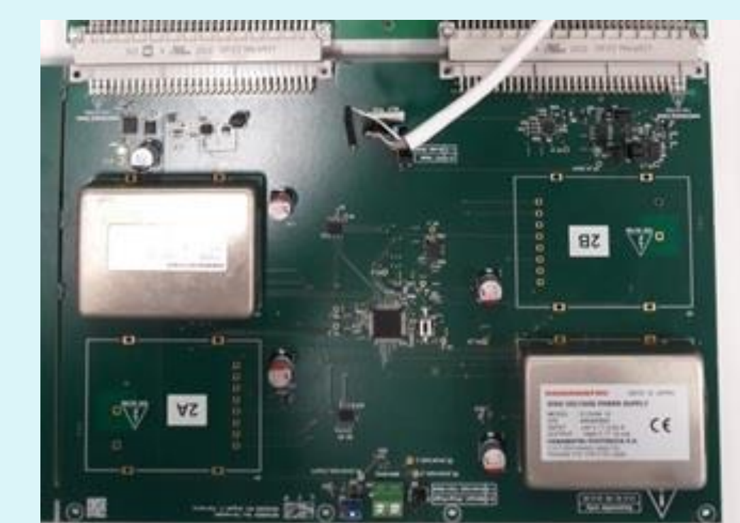
Prototype of the crate for the boards. It has a midplane and the HVremote boards go in the back.
