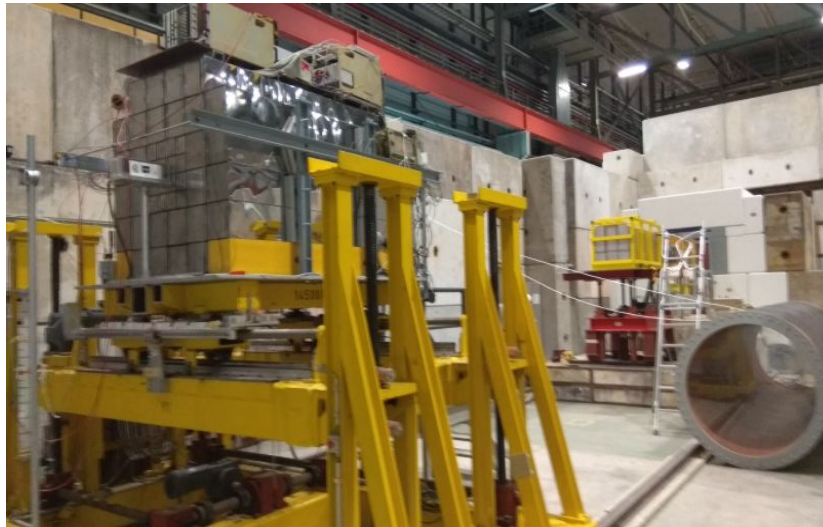
Fig.16. View of the current PSD (close position) and the prototype of the 3x3 modules forward hadron calorimeter FPSD (far position) installed for tests on the NA61/SHINE beamline.
