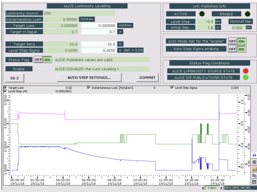
Figure 2: View of the luminosity levelling Graphical User Interface in the LHC_IF WinCC expert application.
