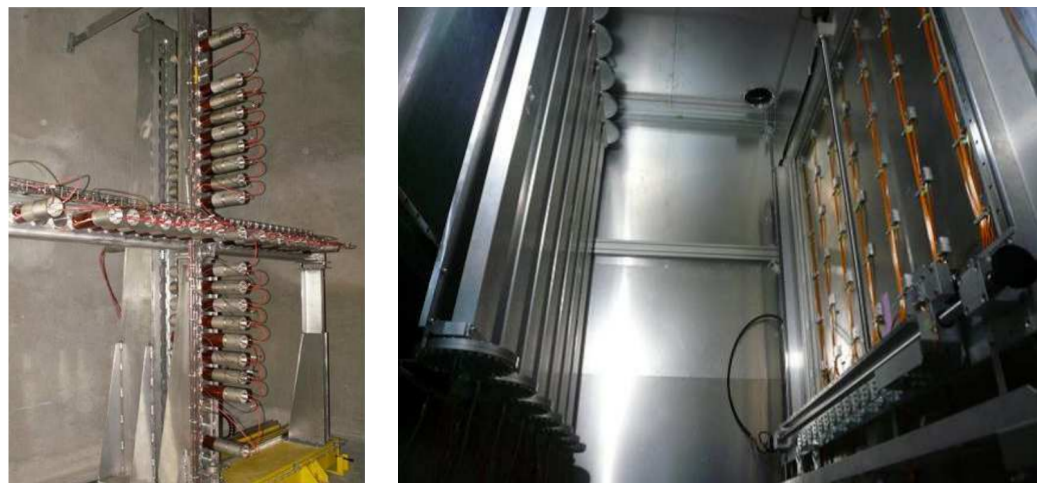
Figure 13. Muon monitoring detectors employed for the CNGS neutrino beam (left) and the J-PARC beam (right). The CNGS chambers consisted of 42 muon detectors separated by 11.25 cm and spanning a length of 2.7 m. The J-PARC system (MUMON) is composed of 7 \times 7 ionization chambers (left side of the picture) and 7 \times 7 , 1 \text{ cm}^2 , PIN photodiodes (right side). The beam enters from the right side. Reproduced under CCA4.0-I license with permission from Sissa-Medialab [28].
