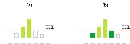
Fig. 4. Illustration of the working principle of the neighbouring-logic. In (a) the situation without NL enabled is shown. In (b) the effect of the NL is shown: even if the signal is too small to surpass the threshold level the neighbouring channels of a signal above threshold are read out as well.
