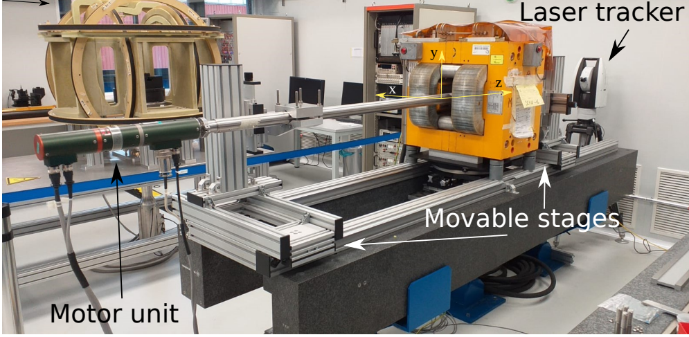
Figure 5: Corrector dipole magnet (yellow) installed on the measurement bench. The motor unit is hosting a stepper motor as well as a rotary encoder.
