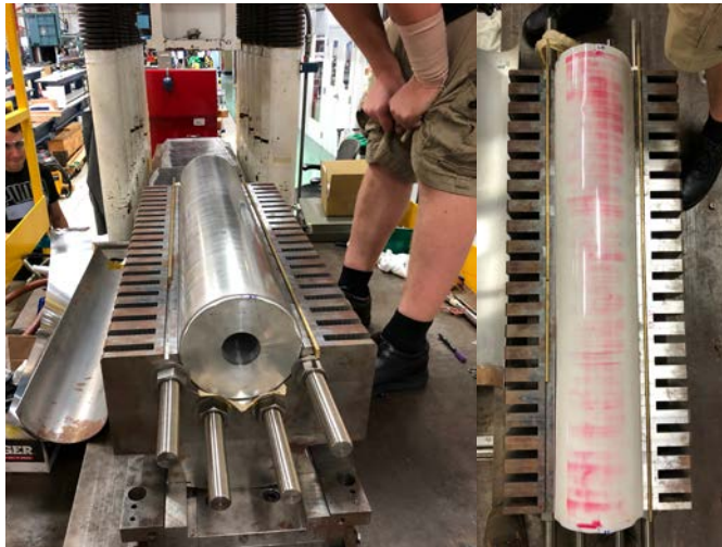
Fig. 9. Axial radial force distribution measured using Fuji film.
