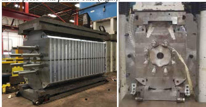
Fig. 8. Long Mechanical Model in between the top and bottom tooling outside (left) and in the press with pusher bars (right).
