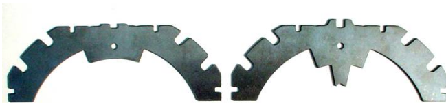
Fig. 3. TQC collar Lamination after (left) and before modifications.
