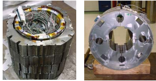
Fig. 10. Assembled Mechanical Model. Collared section shown at left and yoke without collars shown at right.
