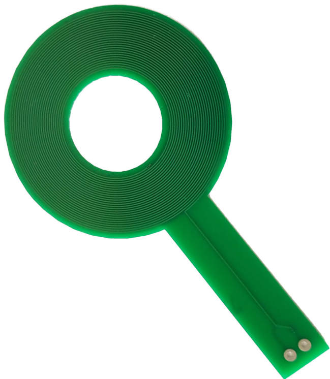
Fig. 1. Detailed picture of a double layered printed circuit board shim coil.
