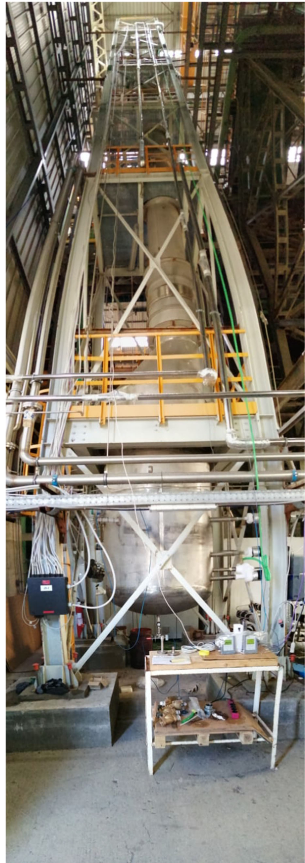
Fig. 10 The prototype Aria plant in the Laveria building of the Carbosulcis mine, Nuraxi-Figus site, viewed from the basis of the column
