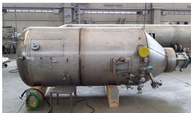
Fig. 5 The bottom module of the column
