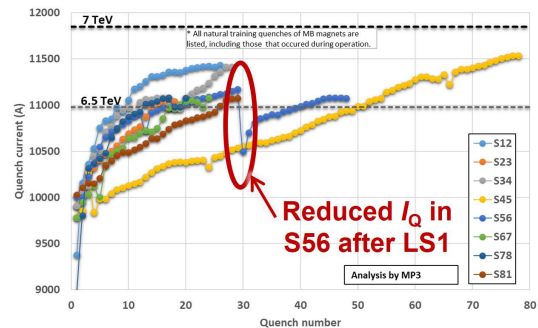
Figure 2: Training behavior of the RB circuits after installation [6].
