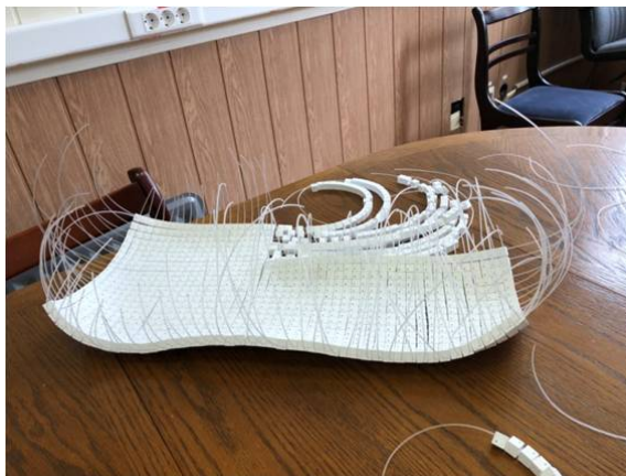
Figure 2. A plane of scintillator cubes formed with fishing lines.
