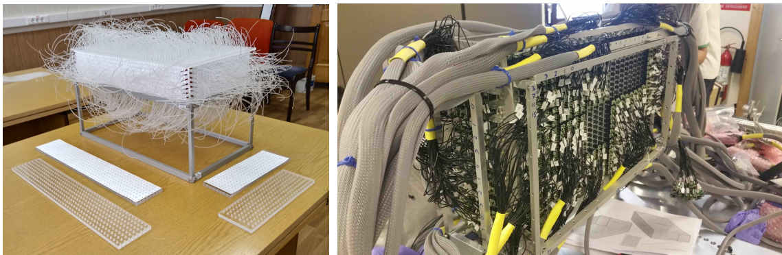
Figure 3. Left: the SuperFGD Prototype volume assembled with the fishing line method, before the insertion of WLS fibers and the attachment of the acrylic box. Right: the partially instrumented SuperFGD Prototype bottom face. The detector is rotated by 90^\circ about the z -axis to enable access to the bottom face.
