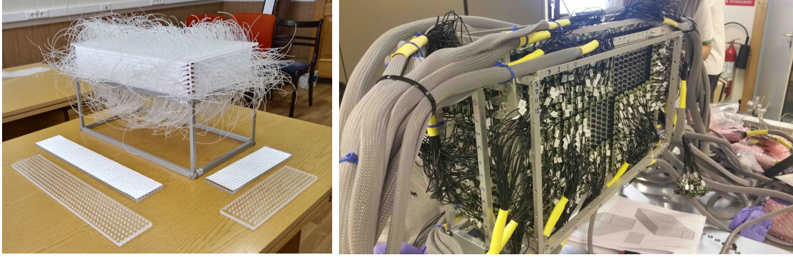
Figure 3: Left: The SuperFGD Prototype volume assembled with the fishing line method, before the insertion of WLS fibers and the attachment of the acrylic box. Right: The partially instrumented SuperFGD Prototype bottom face. The detector is rotated by 90^\circ about the z -axis to enable access to the bottom face.
