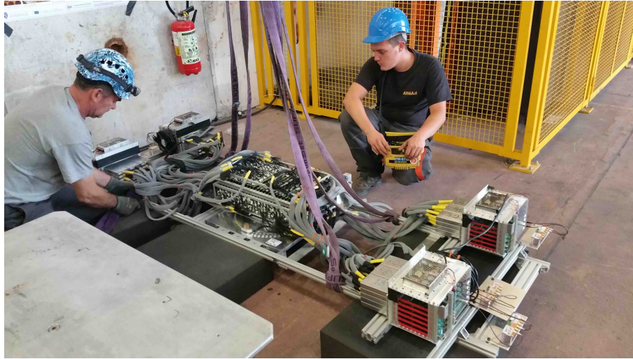
Figure 4: The SuperFGD Prototype in the CERN-PS East Hall during transport to the T9 beamline. The minicrates housing the front end electronics can be seen on each of the four corners of the SuperFGD Prototype mounted in the center of the mechanical assembly.
