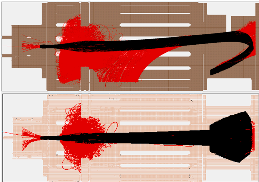
Fig. 19. Simulation of the gauge with SIMION. Electric potential surface for electrons (top) and electron trajectories (black) and ion trajectories (red) from two different views (X and Y as defined in Fig. 17) under nominal potentials. (For interpretation of the references to colour in this figure legend, the reader is referred to the Web version of this article.)
