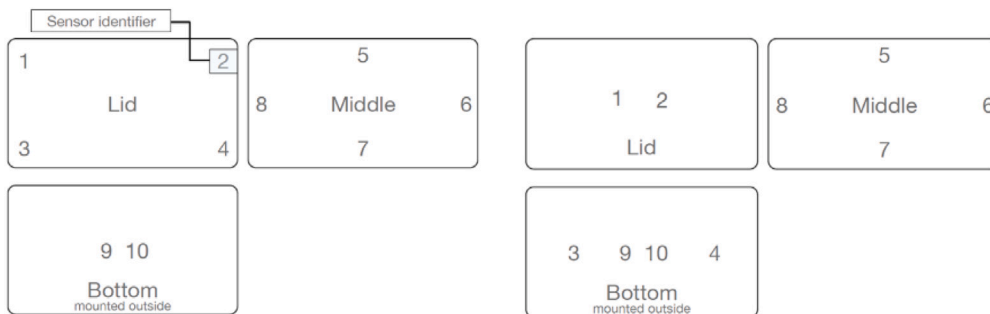
Fig. 5. The two tested geometrical arrangements for a 10-sensor configuration. Left: four sensors at the four corners of the lid, four at the centre of the four side walls, two on the bottom. Right: two sensors on the lid, four at the centre of the four side walls, four on the bottom.
