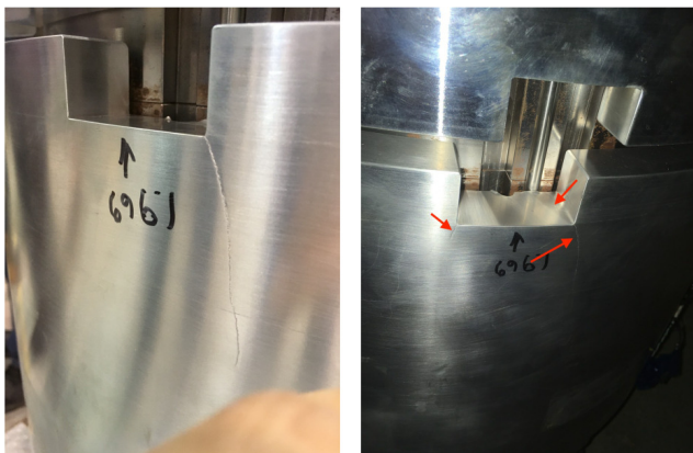
Fig. 4 The other two noticeable cracks on the broken shell: one long crack (left) and the small crack initiated from another corner (right).
