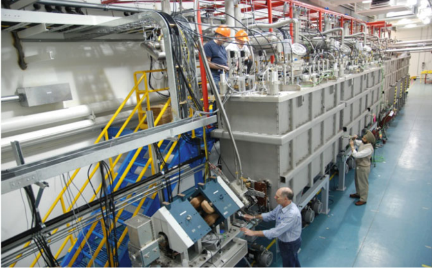
Fig. 11.59 The ISAC-II Superconducting linac. [Courtesy of ISAC/TRIUMF, Vancouver, R. E. Laxdal]
