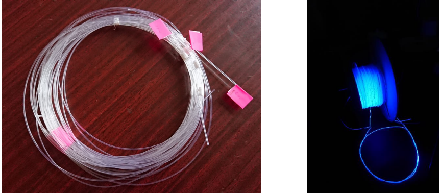
Figure 6: Photographs of the polystyrene-based scintillator filament used for 3D-printing with the FDM technique. On the right picture, the filament was illuminated with UV light.
