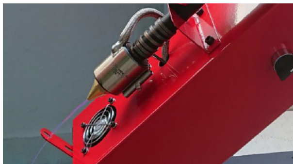
Figure 3: Picture of the extruder used to produce the scintillator filament.
