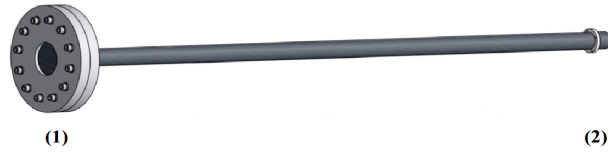
Figure 1.: The T2K replica target with the upstream aluminum flange (1) and the downstream plastic ring (2) used to support the target.
