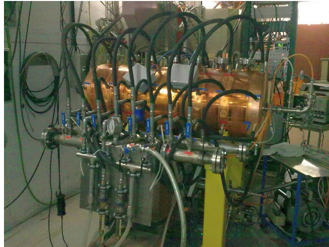
Fig. 2.23: PIMS prototype during the high average power test.
