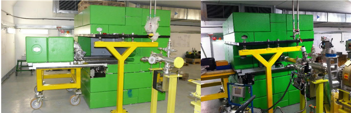
Fig. 3.15: Main dump shielding open for accessing the dump (left) and closed (right).
