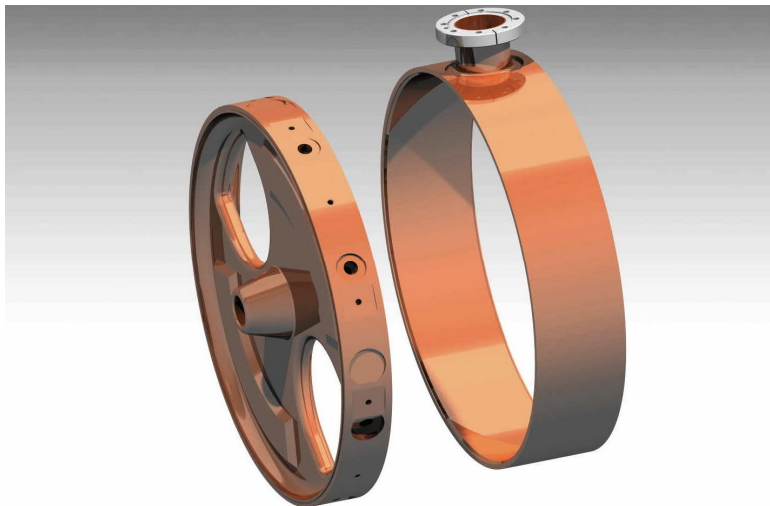
Fig. 2.22: Discs and rings before welding.
