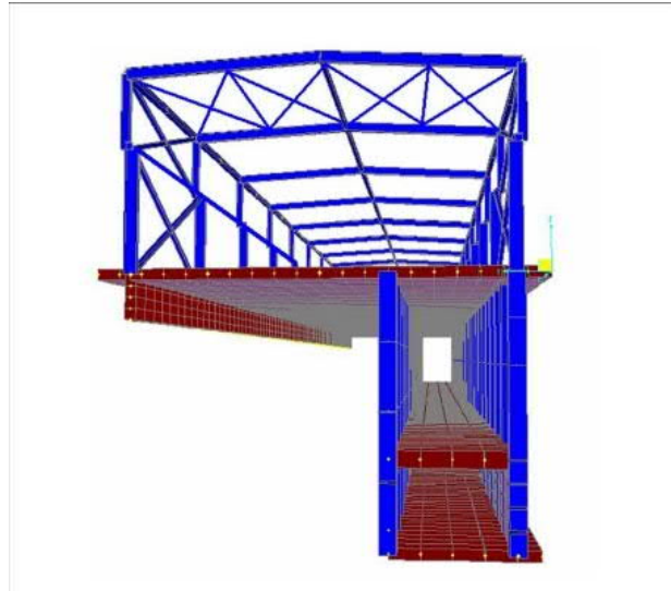
Fig. 4.6: Transverse section klystrons building and tunnel.
