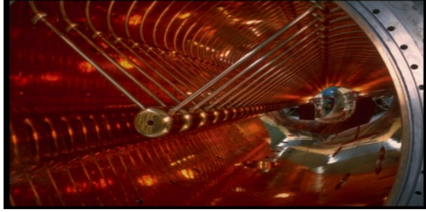
Fig. 7: Unilac at GSI, Darmstadt; the structure of the drift tubes and their increasing length as a function of the particle energy is clearly visible.
