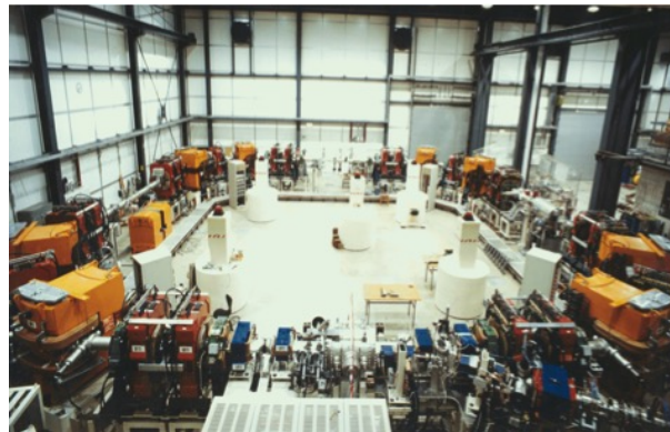
Fig. 12: TSR storage ring, Heidelberg, as a typical example of a separate function strong focusing storage ring.
