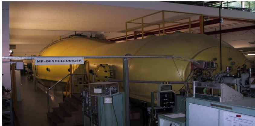
Fig. 4: A typical example of a Tandem-van-de-Graaf Accelerator. These are very reliable machines for precision measurements in atom and nuclear physics. (Photo: Max Planck Institute for Nuclear Physics, Heidelberg)
