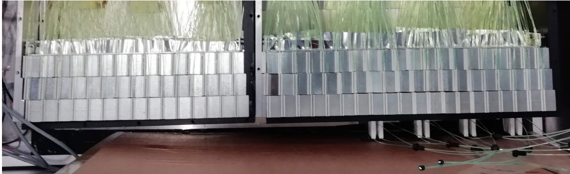
Figure 8: Four doublets of the photon veto installed below Module 3 (bottom rightmost part of the figure).
