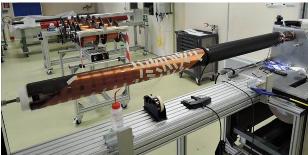
Figure 5. CCT 2.2m winding set up. We see the wire mounted on ten spools, the wire cleaning station where the wires run through felt pads that are loaded with cleaning fluid, and the horizontal winding machine.
