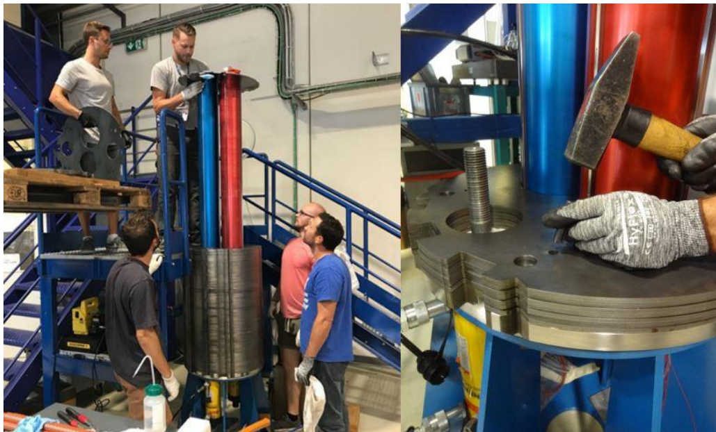
Figure 8. Left: Vertical yoke assembly tool. Right: elastic pin insertion to lock yoke laminations.
