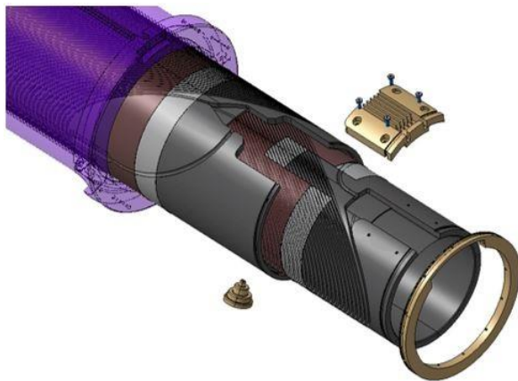
Figure 6. Lead end. We see: the joint box, the outer support collar with flange that fixes the aperture to the yoke at the connection end, the stepped pin that accurately locates the three tubes before impregnation, and the labyrinth ground insulation end ring.
