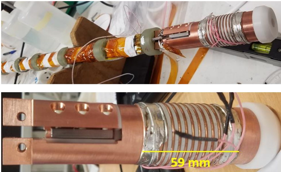
Figure 1. The bottom image shows our VAMAS adapter with a sample mounted before attaching to the measurement probe, shown at the top.
