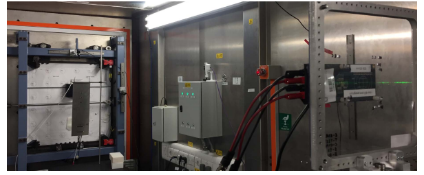
Fig. 7. Irradiation with the SRAM tester at the ChipIr facility.
