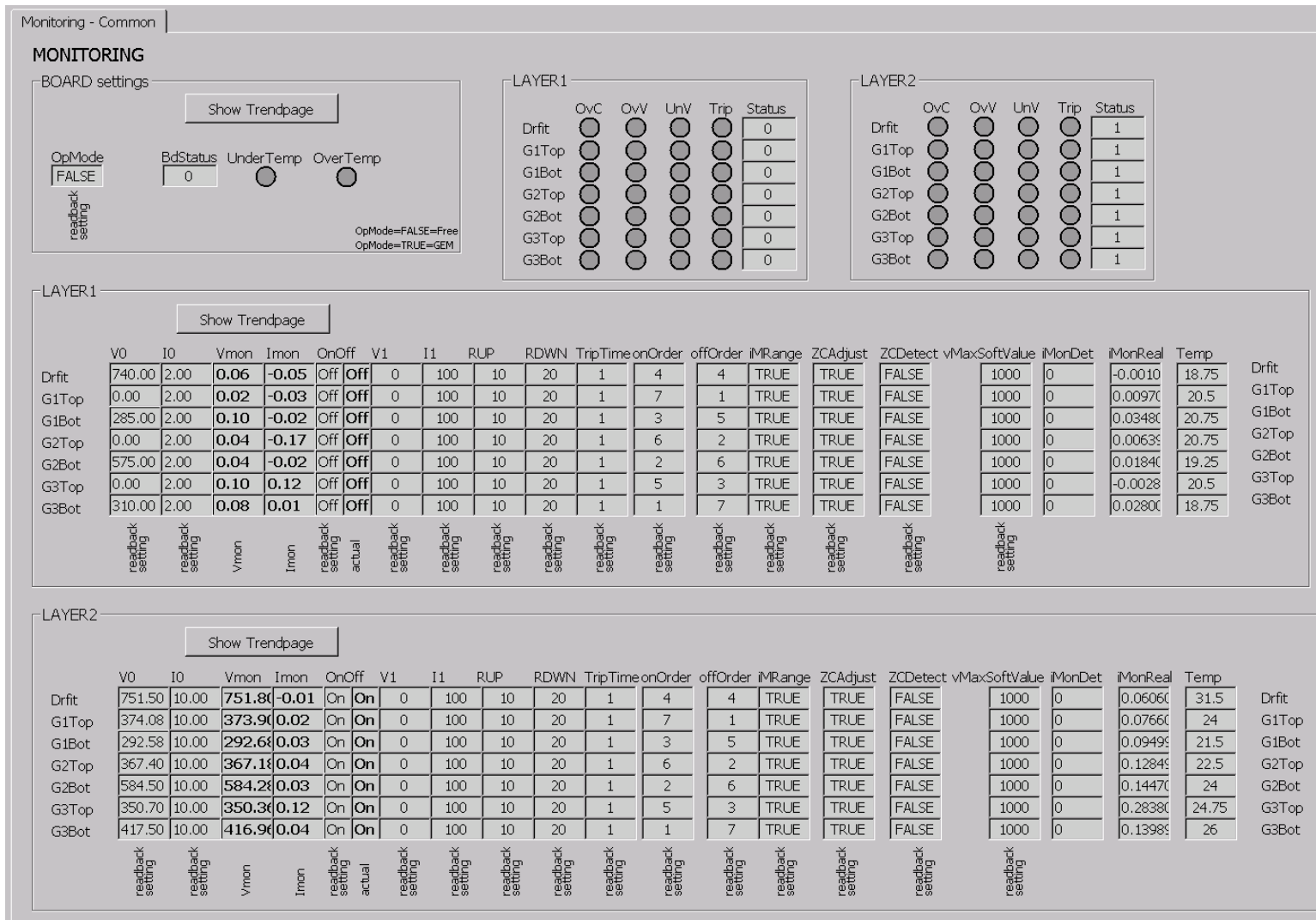
Figure 5. DCS panel for monitoring the actual parameter values of a multichannel power supply.
