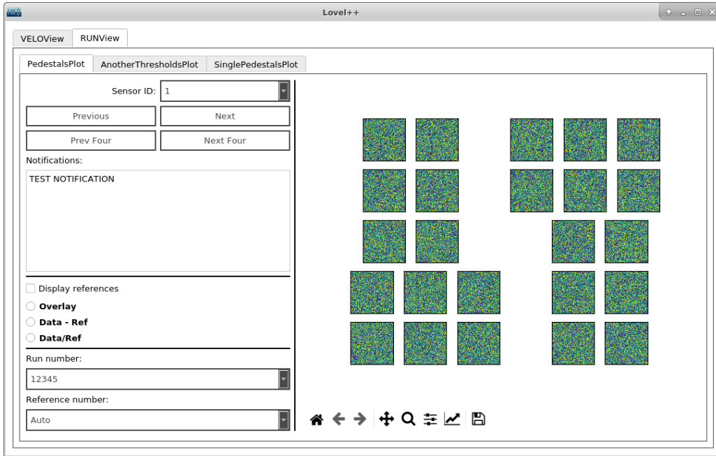
Figure 4. A new version of GUI panel that is part of the new monitoring software platform. The exemplary noise map of two VeloPix parallel assemblies is presented. There is a control panel on the left side that allows switching the view between consecutive VELO sensors.
