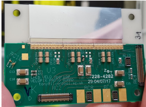
Figure 1. One of the VeloPix sensor triplet prototypes.
