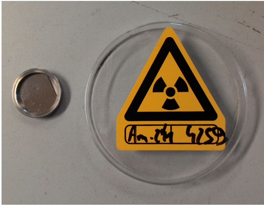
Figure 4. Picture of the the used alpha source.
