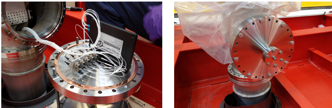
Figure 16. Left picture: DN200CF side of one nibble with a 1 \times 10 splitter (on the right) and a 10-channel patch panel to connect the internal patches to the outputs of the splitter (on the left). Right picture: front view of the DN200CF to DN40CF nibble with a mounted FC/FC optical feedthrough.
