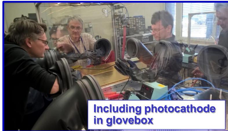
glovebox also to mount the active module onto the RICH
