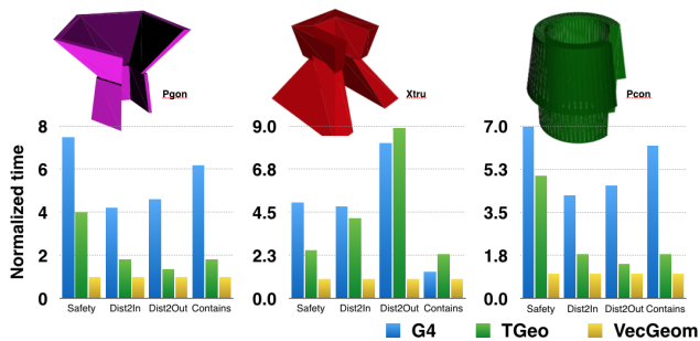
Fig. 9 Performance speedups of more complex primitives (polycone, extruded solid, polyhedron) for scalar interfaces, compared with Geant4 and TGeo. Speedups are averages over all such solids found in the ALICE detector. In these complex cases, no additional basket SIMD acceleration is feasible.
