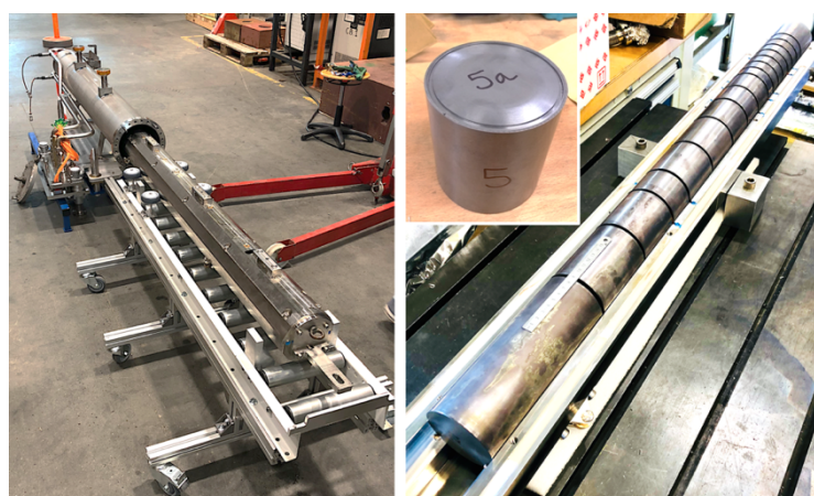
Fig. 5. Photos of the target prototype assembly being prepared for final installation. The right part shows the internal cladded blocks with the gaps between each other corresponding to a 5 mm gap required for the water cooling of the target assembly.
