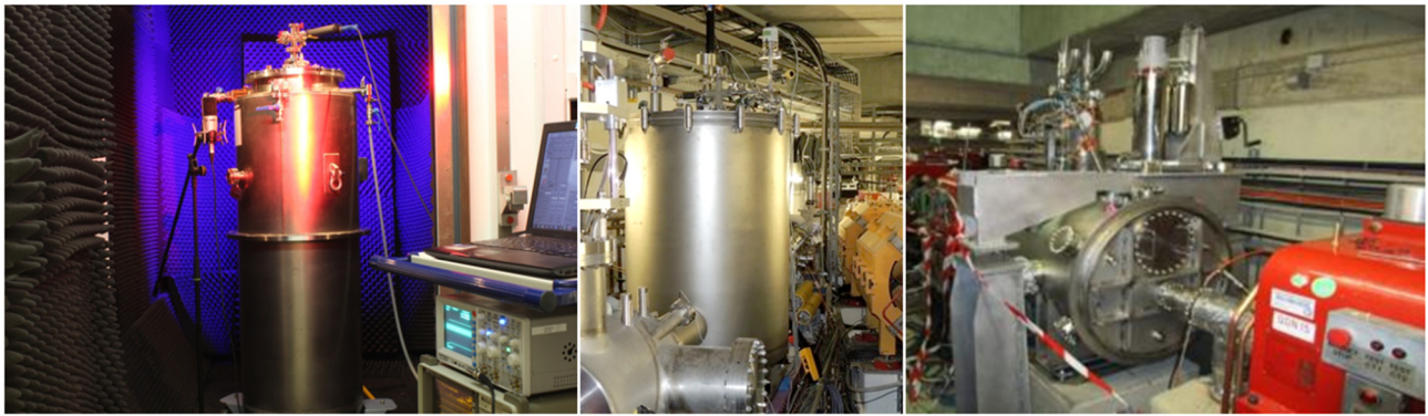
Figure 2: Wide-neck bath cryostat in an acoustically and magnetically shielded chamber for the electrical CCC-testing at the Cryo-Detector Laboratory at the University of Jena (left), beamline cryostat of the GSI-Pb-CCC at GSI Darmstadt (middle), beamline cryostat and He-reliquefier of the CERN-Nb-CCC at CERN-Antiproton Decelerator (AD) (right).
