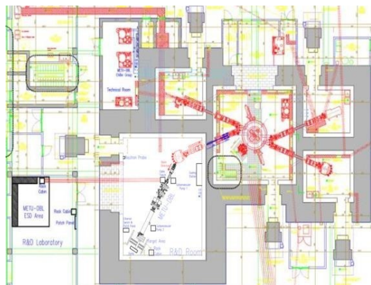
Fig. 1. The schematic design of TAEA SANAEM Proton Accelerator Facility. The cyclotron is seen in red on the right, where 4 arms extend out to 4 different irradiation rooms. The one on the lower left is the R&D room in which METU-DBL is shown in black. The connection between this R&D room and the control system in the R&D laboratory is provided by the underground trench shown here in red.
