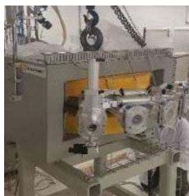
Fig. 11. 5-port magnet installed in the R&D room of the TAEA SANAEM PAF. METU-DBL beamline follows from the right-most exit of this magnet.
