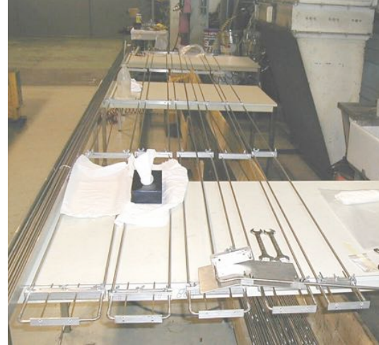
Figure 7: A few steps of the procedure to glue straight and U-shaped tubes.
