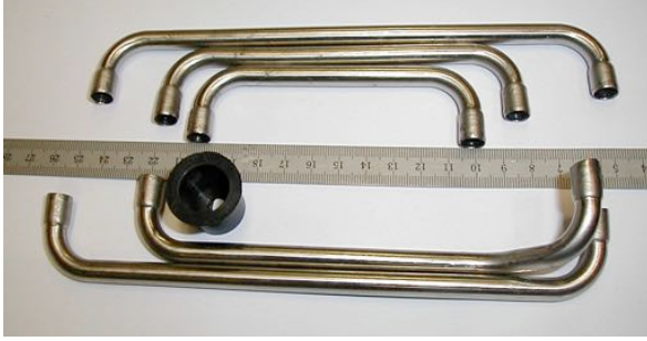
Figure 6: Examples of U-shaped tubes. The rubber cap is used to protect the calorimeter tiles from light, dust and glue during the interconnection of the tubes.
