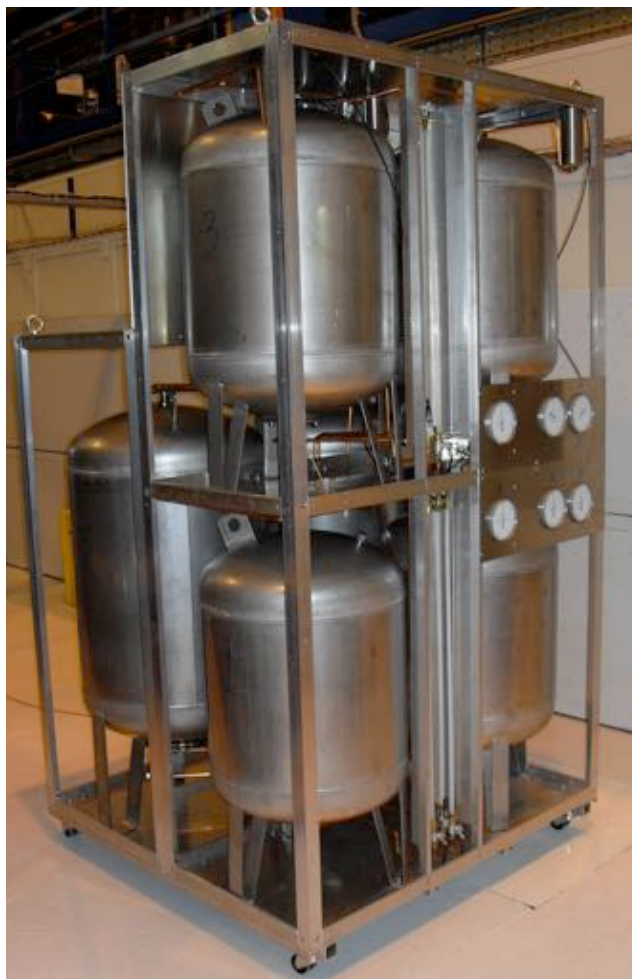
Figure 16: Liquid storage unit, made of two 230 l and four 130 l stainless steel tanks combined in pairs, for the liquid and air volumes.
