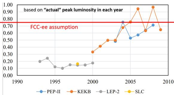
Figure 9: Efficiency calculated from a typical peak luminosity in each year: actual peak in that year (LEP), peak reduced by ~15% (SLC, PEP-II), average of the daily peak luminosity over the year after removing values below 10% of the peak (KEKB), and design value (well defined, FCC-ee).
