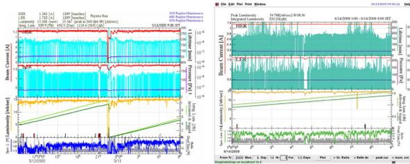
Figure 8: Example evolution of KEKB beam currents and luminosity in 2005 [18] (left) and in 2009 [19] (right). Stored beam current of HER (red line in the top figure), LER (red line in the middle figure), and luminosity (yellow line in the bottom figure) of KEKB over 24 h.
