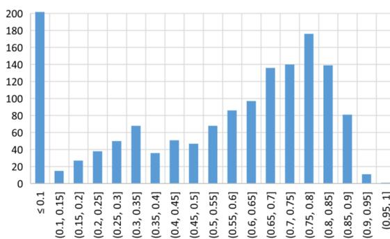
Figure 13: Histogram of KEKB day-by-day efficiency values in units of fraction for the time period with top-up injection, from 2004 to 2010; including shutdowns, technical stops, beam commissioning periods, and machine studies.
