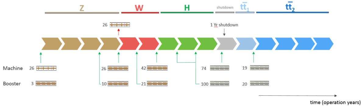
Figure 1: FCC-ee operation time line. The bottom part indicates the number of cryomodules to be installed in the collider and booster, respectively, during the various shutdown periods.
