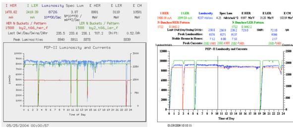
Figure 7: Example evolution of PEP-II beam currents and luminosity in 2004 [17] (left) and 2008 [12] (right). Stored beam current of HER (red curve), LER (green curve), and luminosity (blue curve) of PEP-II over 24 h.
