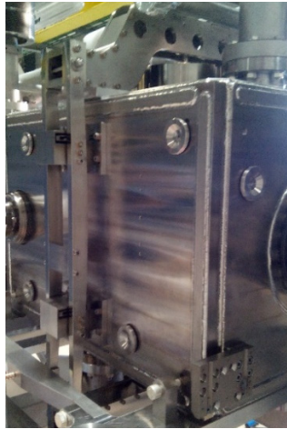
Figure 4: Tuning frame and flexural guides on the DQW helium tank.
