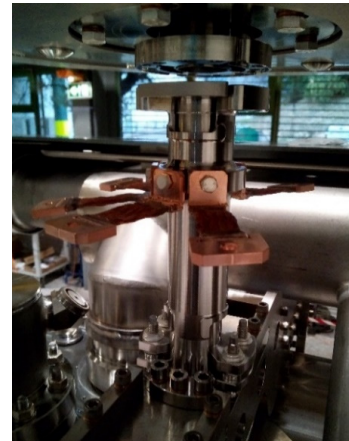
Figure 6: The concentric tuning tubes with thermalisation.
