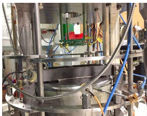
Figure 6: Upper wafer in its support, facing the cavity.
