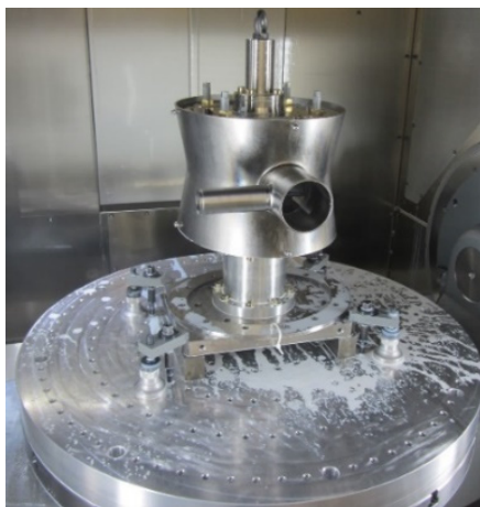
Figure 3: DQW crab cavity subcomponent during machining, with an optimized clamping system.
