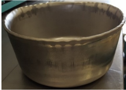
Figure 2: DQW crab cavity subcomponent before first machining, after the deep drawing process. See wrinkles on the top side.
