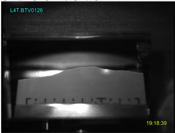
Fig. 4. Image from the radiation-hard camera of the broken BTV screen. The foil holder, ready to be put into beam position, can be seen at the right behind the screen. The glow on the top edge, right from the centre of the screen, is the position of beam impact previous to breakage.
