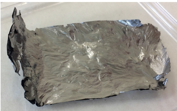
Fig. 8. DLC-23-1000-S foil that was detached from the foil without being tested with beam. The hypotheses is that the frame of this foil was hit by the showers of particles produced by mis-steered beam hitting the machine aperture, just upstream of the loader, during low energy tuning of the linac.
