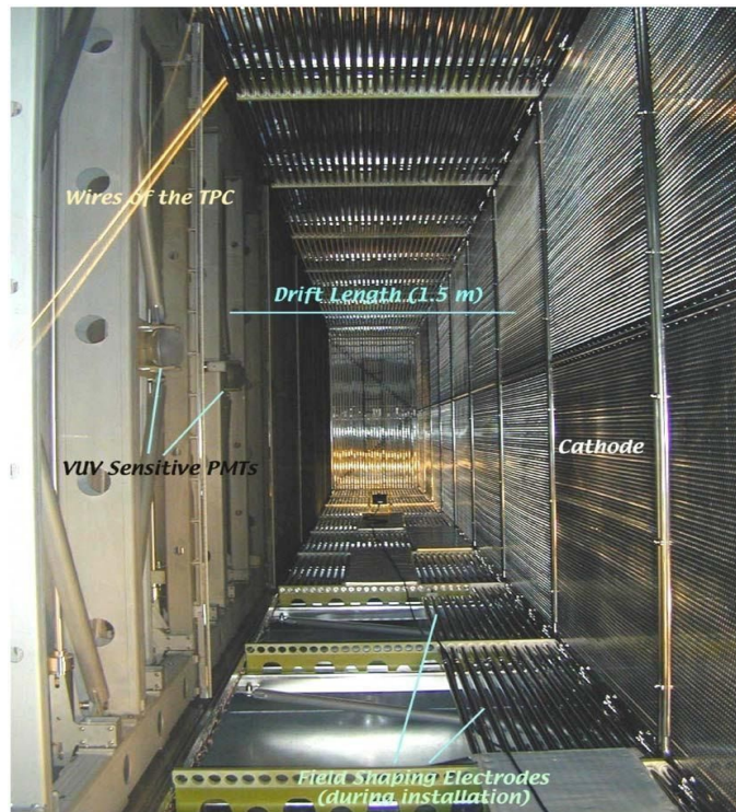
Figure 1. Cross section of ICARUS detector TPC during the assembling in Pavia, showing the field shaping electrodes, the cathode, the anodic wire planes and the PMT system.
