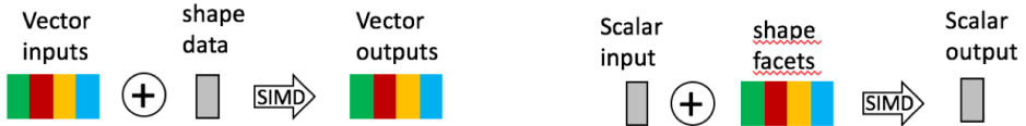
Figure 1: VecGeom is exploring different vectorization paths. The throughput can be increased by operating on multiple input data with SIMD operations (left) or by executing faster single queries vectorizing on internal loops over faces (right).
