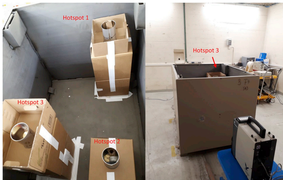
Fig. 8. Description of one of the experiment configuration. Left picture: inside the container, sources are located in tin cans. Right pictures, measurement configuration with FALCON detector.
