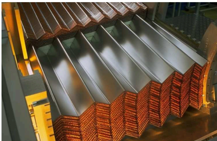
Picture of an electromagnetic end-cap module during stacking, showing the accordion structure of the ATLAS EM calorimeters.
