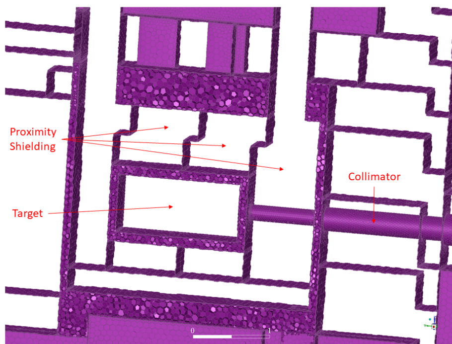
Figure 2. Mesh slice in the collimator-target region, showing the gaps between the target and the shielding blocks.
