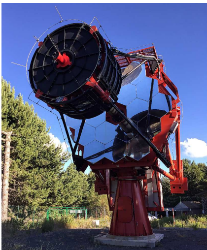
Fig. 1. ASTRI-Horn dual-mirror Cherenkov telescope installed on Mt. Etna (Italy) at the INAF M.C. Fracastoro observing station.
