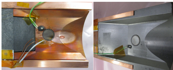
Figure 8: Jaws downstream taperings in Glidcop (left) and in MoGr (right).
