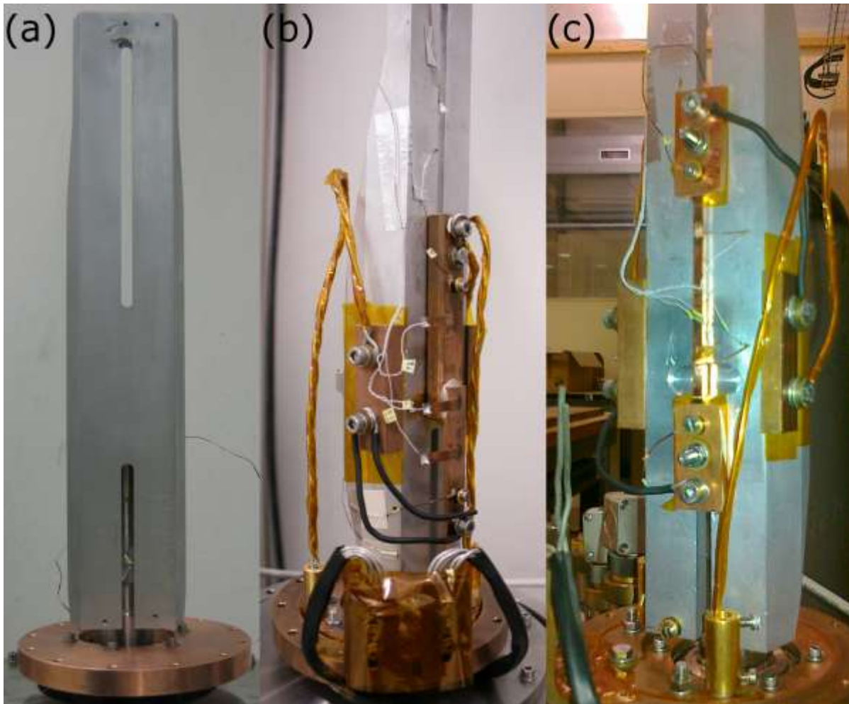
Figure 7: Sample holder with (a) no instrumentation or sample, (b) instrumented lap-splice sample with two Cu-wires per side for current input and (c) instrumented butt-splice sample with one Cu-wire per side for current input.
