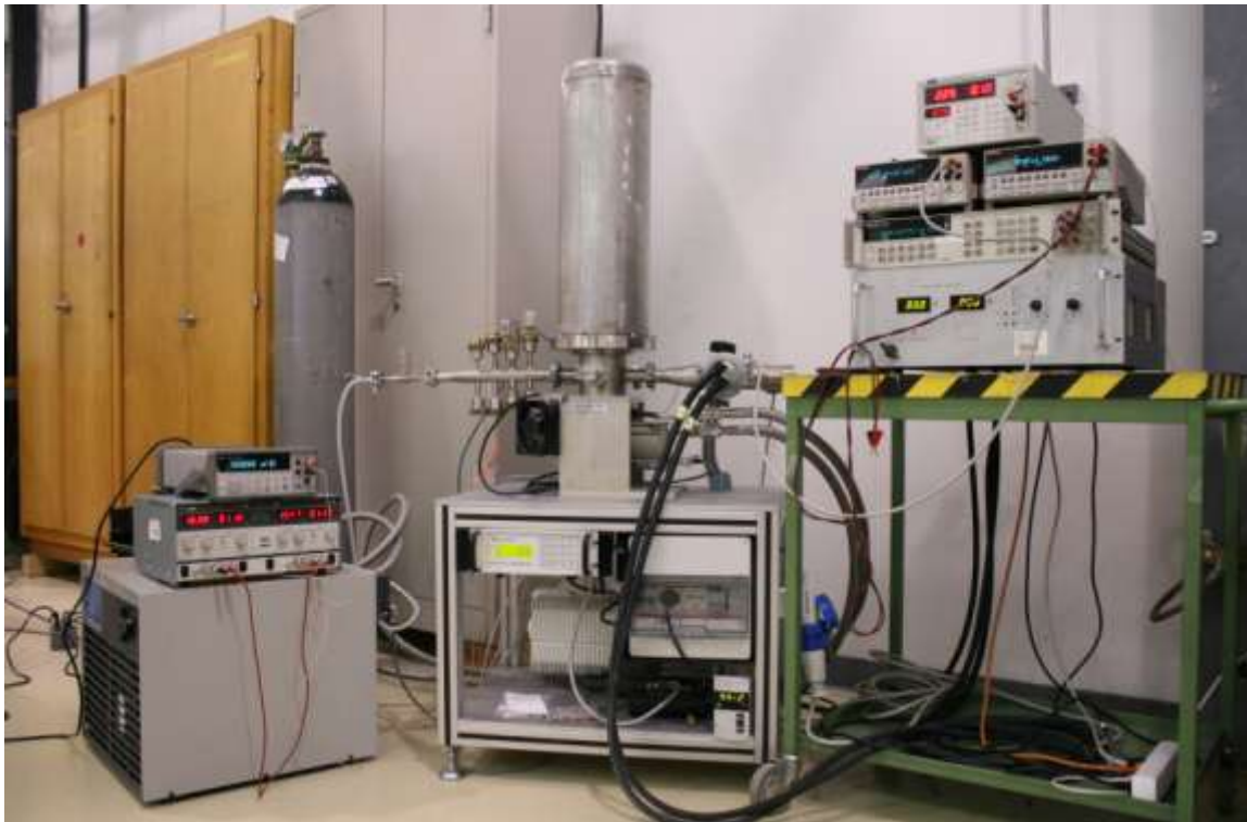
Figure 5: The modified cryocooler setup.
