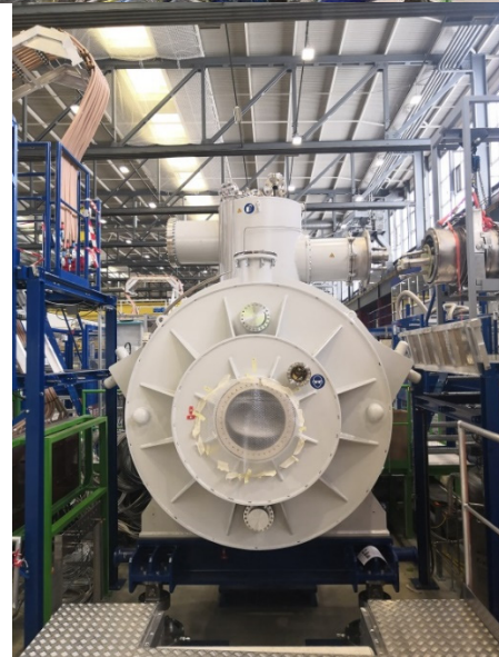
Figure 4: Top: Test bench overview. The three test benches (coloured blue, green, and white) can be seen. Bottom: short multiplert on test bench. On the left hand side are the power cable connection, on the right hand side the connection to the cryogenic jumper line.
