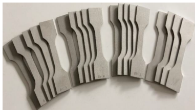
Figure 1: The specimen produced by the '3D Metal' project to measure the tensile strength of additively manufactured parts produced on different machines with different technologies and different parameters.
