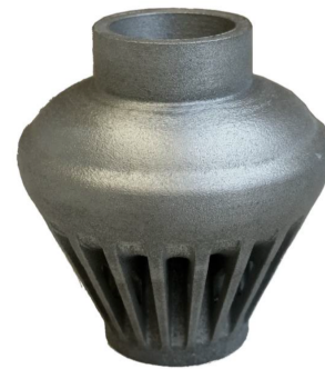
Figure 7: A 6 GHz Niobium cavity built in two manufactured at CERN using additive manufacturing (Source: Romain Gérard, CERN).
