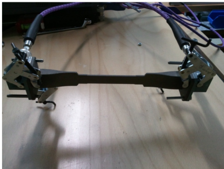
Figure 6: Measurement of the RF parameters of a waveguide buyilt using additive manufacturing (Source: Alexej Grudiev, CERN, https://indico.cern.ch/event/275412/ ).
