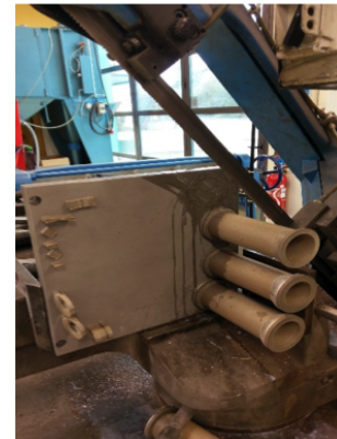
Figure 3: Beam pipes on their manufacturing support, right after they were printed using selective laser melting (SLM). Before being used the pipes had to be sawed off their support (the saw can be seen on the top right corner of the image) and the knife-edge improved with a lathe. Image taken from [2].
